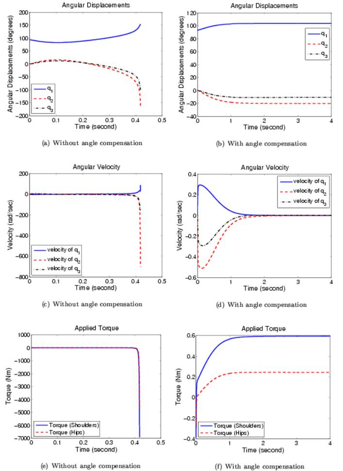
Figure 12: Simulation using Linear Quadratic Regulator for balancing without and with angle compensation
