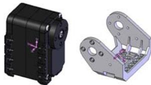
Figure 8: 3D models of a servo and a component of the humanoid robot showing the centroid and the principal axes of the moment of inertia tensor.
