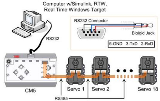
Figure 2: Humanoid control architecture
