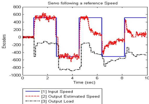
Figure 3: Servo following a reference velocity with open loop velocity control
