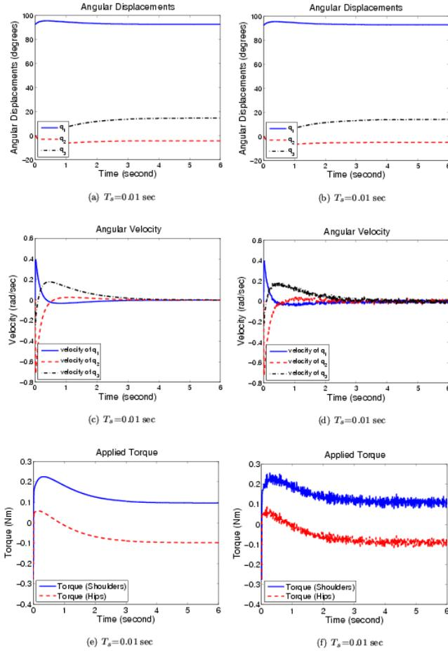
Figure 13: Simulation using angles compensation for the three joint and simulation corrupted by servos position resolution
