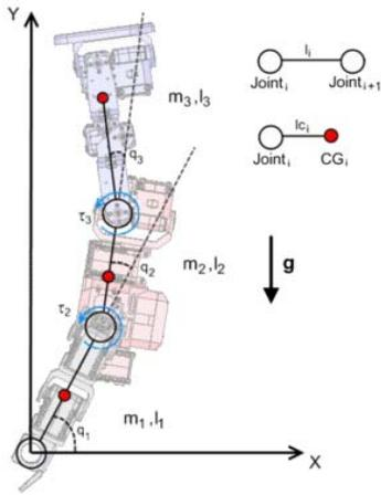
Figure 11: Representation of the humanoid robot seen as an underactuated 3-link inverted pendulum.
