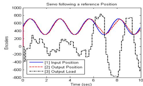
Figure 2: Servo following a position (close loop control)
