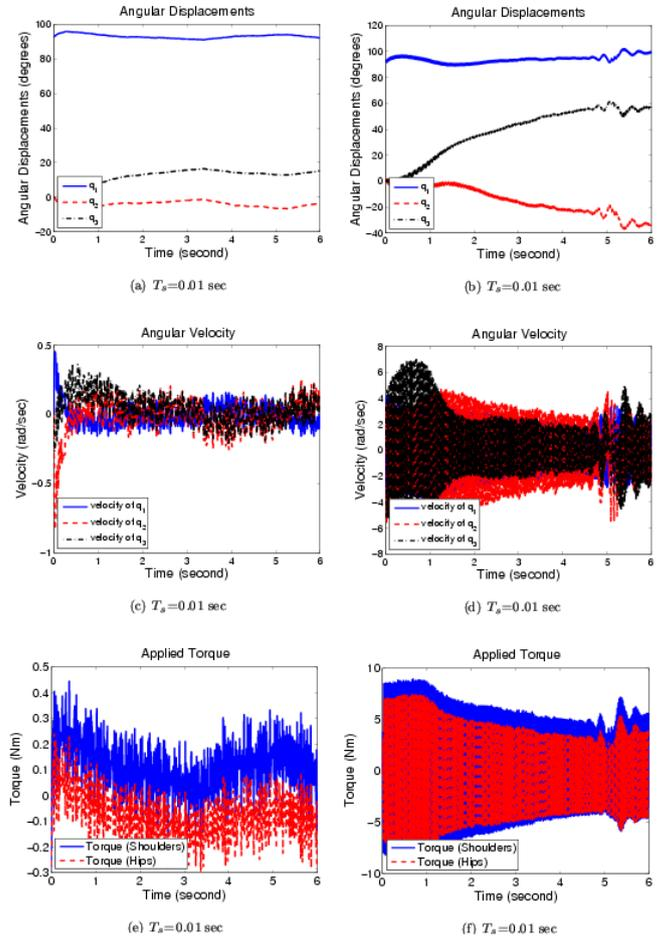
Figure 14: Simulation after adding gyroscope resolution and simulation with dead-zone response of the servos
