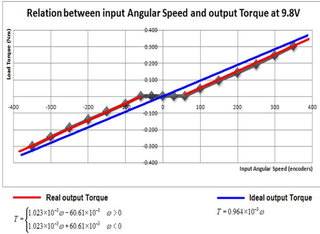
Figure 7: Speed to Torque Relation
