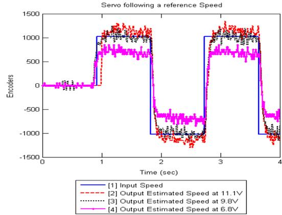
Figure 5: Effects of the supplied voltage to the servos in the outputs velocity response
